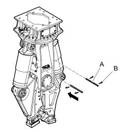
The piston rod sheaths are now prevented from slipping out.
