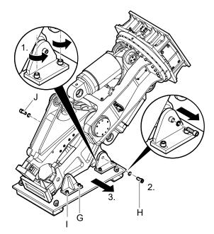
Lift the hydraulic demolition cutter.
