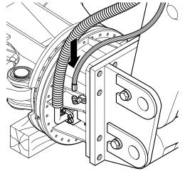
Connect both hoses for the function »Turn« at the boom in a torsion-free manner.
