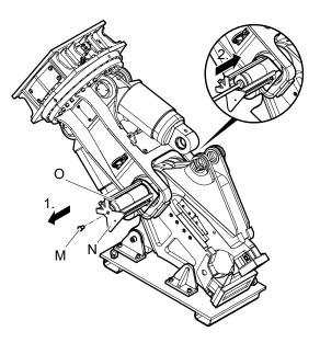
Disassemble the bolt cage (N).
