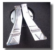
**TRAVEL CONTROL**Dual hydraulic transmission foot controls are more responsive and comfortable for operator comfort.
