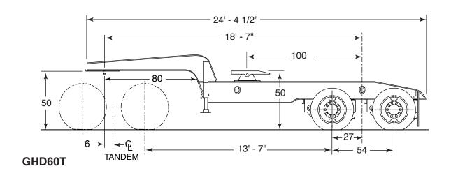
Capacity: Proportionate share of up to 60 tons Minimum trailer gooseneck clearance radius - 168"
