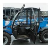
Fully Enclosed Cab Increase operator comfort and decrease fatigue in a clean, dry, quiet cab with standard windshield washer, as well as a heater and defroster for cold climates. Front window doubles as an emergency exit. Left and rear windows open for ventilation. Air conditioning is also available as an option.
