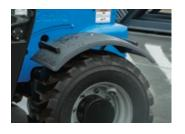
Fenders are also standard keeping the machine cleaner as well as shields the operator from mud being slung.
