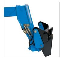
Universal Skid Steer Adapter This option allows you to pull up and attach to a wide variety of skid steer type attachments in just seconds, reducing your overall equipment costs and increasing the versatility of your fleet (GTH<sup>™</sup>-5519 only).
