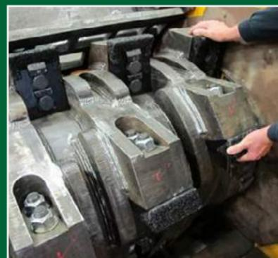
Segmented drum rotor with brute package has twenty striker plates held in place by two 1-1/4" bolts, designed for contaminated demolition debris, railroad ties, and MSW. Striker plates, edged with aggressive carbide, pulverize material and outlast with impressive durability, saving time and money. Striker plates pictured to the right.
