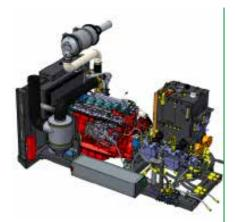
A powerful Scania engine with a low operating speed combined with an efficient hydrostatic drive creates a very responsive shredding action with protection against unshreddable contaminants
