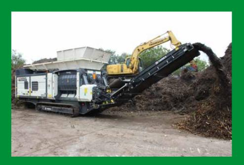
The TDS V20 screen system which is available in different sizes, comes complete with an intelligent protection system, allowing a desired particle size to be produced, whilst still being able to cope with foreign objects.
