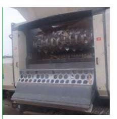
Medium speed shredder with aggressive cutting teeth Intelligent tramp protection system
