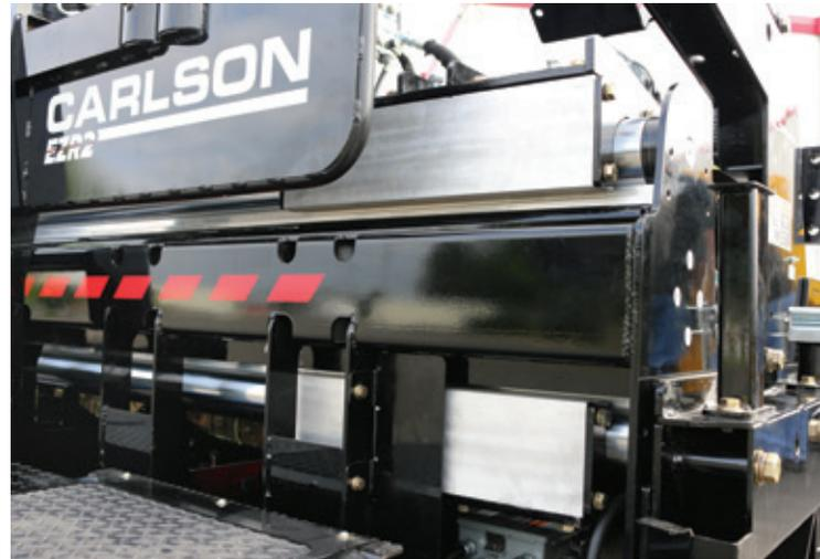
*Featuring a class-exclusive extension support system and oversized adjustable slide blocks, the EZR2's extensions eliminate flex and allow contractors unmatched wide width paving ability.*
