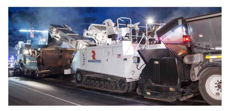
The MTV-1100e and MTV-1105e share the same material handling, frame structure, and controls. Experience Roadtec's famous performance on wheels or tracks.
