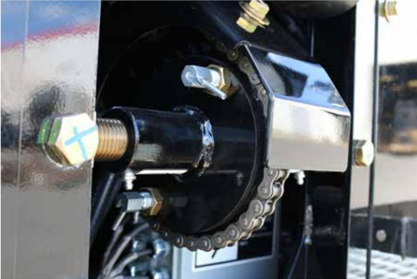
The EZV features a heavy duty, machined power crown assembly with pull pins for adjustment of the lead crown.
