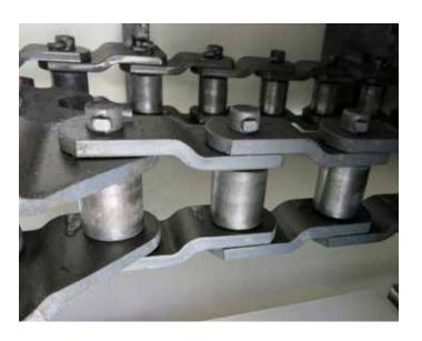
Roadtec conveyors are outfitted with offset durable roller bushing chains.
