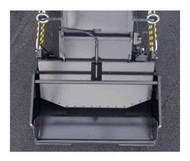
Sized for mass discharge from standard haul trucks, the front hopper allows trucks to unload fast. A steep slope and vibrating bottom plate prevent material build-up.
