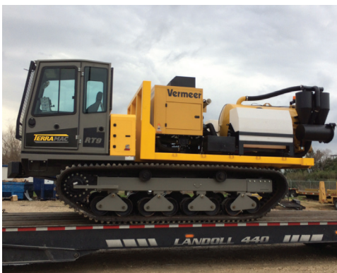
Vacuum Excavator Unit
