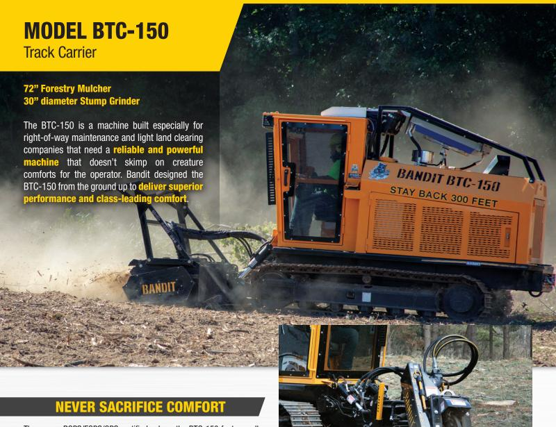
The roomy, ROPS/FOPS/OPS certified cab on the BTC-150 features all the trimmings to keep an operator comfortable during the long days of grinding and mowing. Ballistic-grade polycarbonate glass provides a superior view of the mower or stump grinder, and a thermal insulation reduces outside noise while keeping the inside guiet and regulating the temperature.
