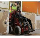
THE REACH YOU NEED Industry leading 81" hinge pin height while maintaining 515 lbs. rated operating capacity.
