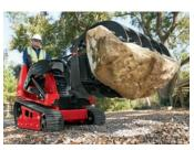
UNMATCHED STRENGTH Vertical lift loader arms allow the TX 1000 to lift and transport heavy loads with a rated operating capacity of 1,000-plus pounds.
