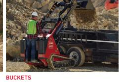
Perfect for light-duty grading, leveling and material handling. Buckets vary in capacity from 4.3 cu. ft. to 9 cu. ft. for lighter materials.
