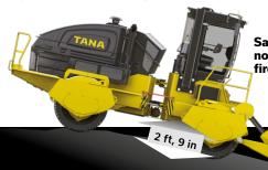
Safe design without belly pans: no debris accumulation to cause any fire hazards.
