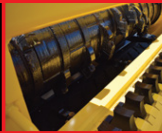
Hard weld surfacing to prolong the life span of the rotor tube.
