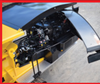
Swing out doors allow easy access to power pack.
