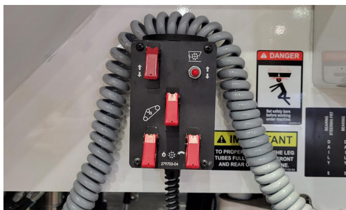
A magnetic-based pendant control box provides access and easy operation while under the machine.
